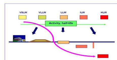
Fig. 1: Increasing Levels of Waste Isolation
