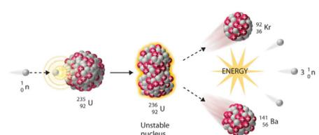
Figure 2. Two examples of fission of uranium – 235 atom
