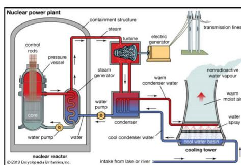
Figure 1. Schematic of a Nuclear Power plant
